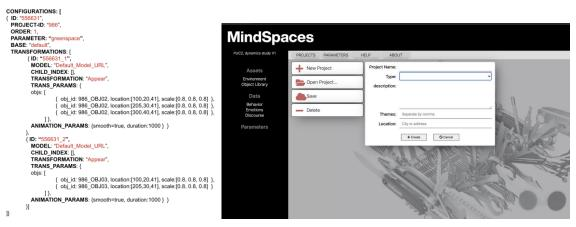
Figure 39 Design configuration editor and resulting JSON
