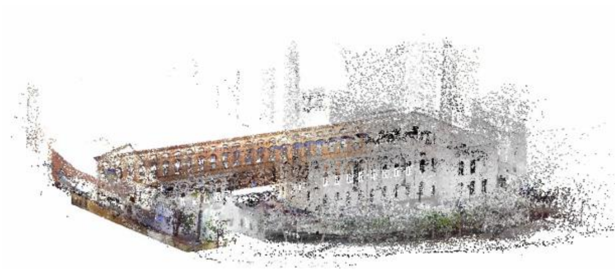
Figure 59. Final dense pointcloud from the Tecla Sala 3D survey (SfM)
