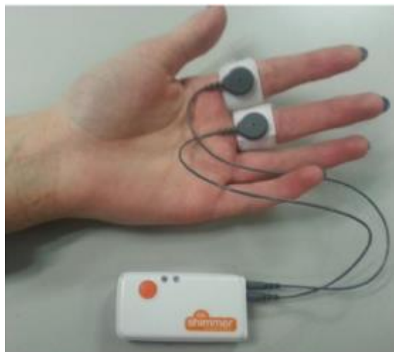
Figure 26. Electrode positioning for GSR
